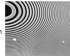
Zone plate x-ray "lens" Outer ring spacing ~35 nm
